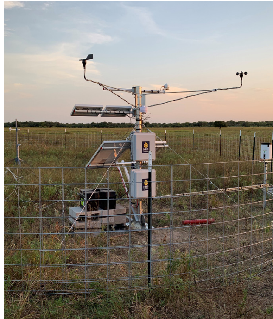
A photo of an NRG Solar Resource Assessment (SRA) station installed for a resource assessment campaign. SRA stations will measure solar radiation, wind speed and direction, soiling, rainfall, temperature, pressure, and humidity for a given location. All these measurements are used to accurately determine solar resource availability before developing and deploying a solar farm.
