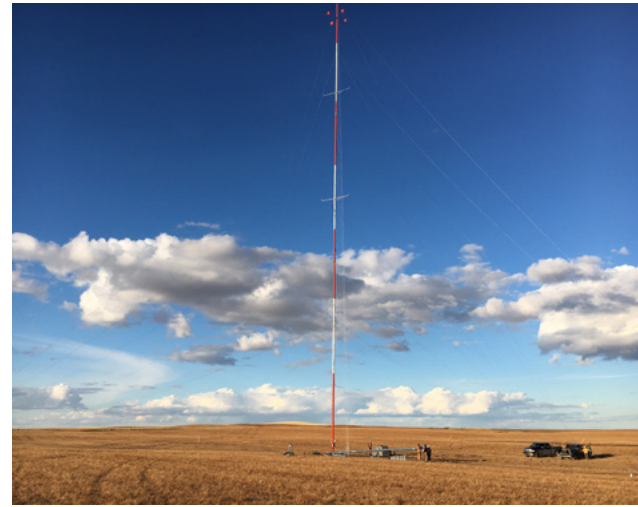
An NRG wind mast installed for a wind resource assessment campaign. These masts are typically left in the field to collect data for 24 months. The data determines the potential energy production for the site being assessed.
